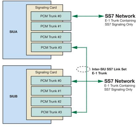
Figure 17. Inter-SIU Link over Crossed E-1/T-1 Cable
